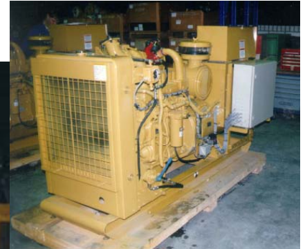
(Above) The 3304 DIT generator set with EMCP and secondary shutdown system
