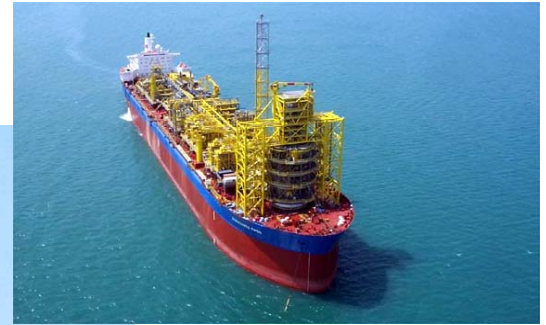
(Above) Espadarte FPSO with completely renewed top sides on its way from singapore to the Espadarte field. You can see the 5 gas compression units behind the turret.
