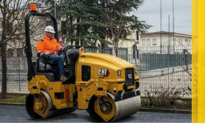
The Cat® GC 2-3 ton utility compactors are well suited for a variety of applications from asphalt work to base compaction and even landscaping. They are designed with industry leading features and performance to get the job done.
