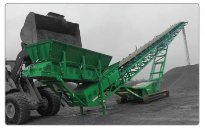
HIGH CAPACITY HOPPER Over 7 cubic yards allows for larger amounts of material to be directly loaded into the hopper.
