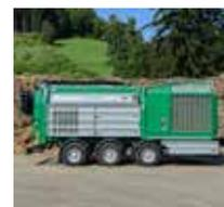
The mobile Terminator gives you the choice between hook, three-axle trailer or tracked versions. On the hook version, a towing facility provides manoeuvrability at the site. The trailer version has air-cushioned axles and positioning capability for comfortable mobility. The tracked version with two-stage drive and extra-wide treads is mobile on unhardened surfaces.
