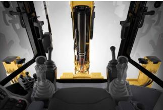
The 444F2 is fitted with Pilot controls providing low effort operation, with the ability to switch between ISO (Excavator) or SAE (Backhoe) control patterns with the press of a button. Providing easy and safe operation for operators of any experience or ability.
