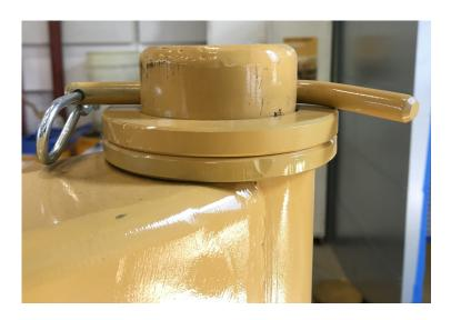
Joint lowers throught the swing arms from top. Install plate bottom and secure with bolts, washers, nuts and locker pins.
