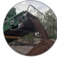
**FINES CONVEYOR** 48" Fines conveyor features heavy duty underside impact rollers, spring loaded adjustable belt scraper and built in pressurized dust suppression.
