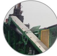
**RADIAL RETURN CONVEYOR** Features full length dust suppression control, and allows operators to recirculate oversize material from the screenbox back to the feed hopper or radial a complete 90° while running.
