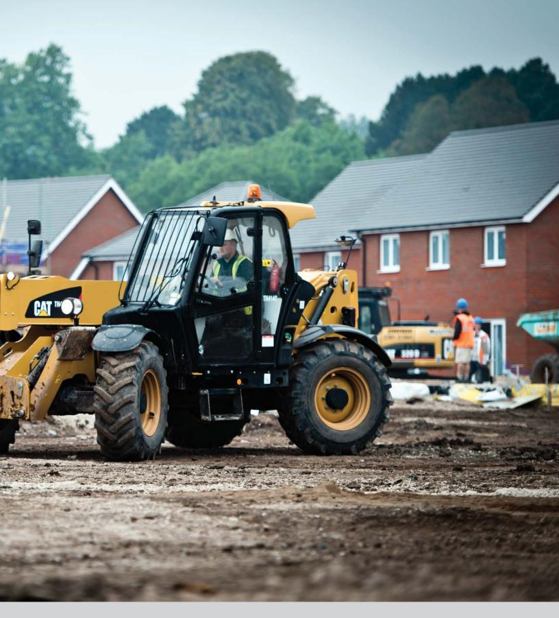
The C Series Telehandlers have a new engine to meet EU Stage IIIB equivalent emission standards and a new powershift transmission that ensures the operator can easily select the right ratio for the job in hand.
