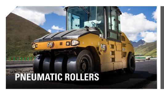
Cat pneumatic compactors offer a wide range of operating weights to meet specific application needs. Steel, sand, and water provide versatile ballast options.
