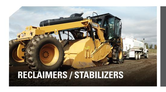
Cat road reclaimers/soil stabilizers pulverize the asphalt layer and mix it with the underlying base or mix additives and aggregates into the soil to stabilize deteriorated roadways or soil for a strong base.
