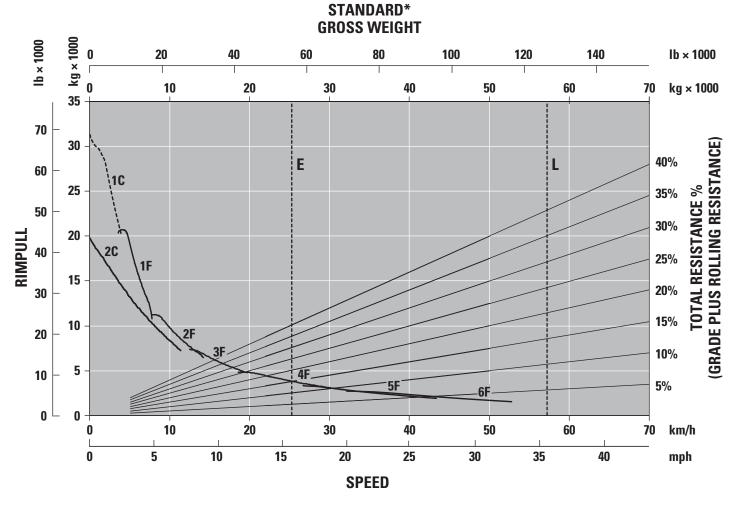
1C – 1st Gear (Converter Drive) 1F – 1st Gear (Direct Drive)
