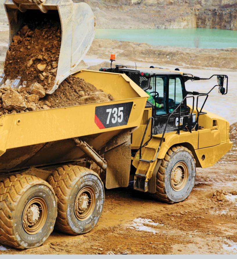
The Cat 735 with a 20 m<sup>3</sup> (26.2 yd<sup>3</sup>)/32 tonnes (35.3 tons) capacity, offers demonstrated reliability and durability, high performance and productivity and a new world-class cab to improve operator comfort and ease of operation.
