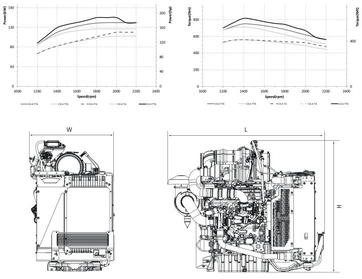
The above dimensional drawings are based on the turbocharged aftercooled model
