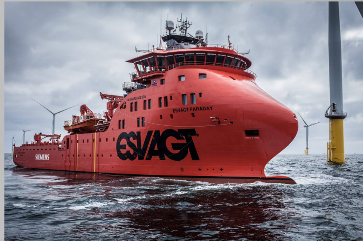
Esvagt Faraday, equipped with 4x 3516C Variable speed genset engines, 1771bkW, 900-1600rpm.
