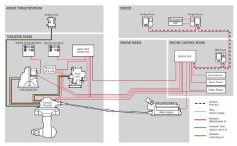
If space is insufficient, the header tank can be replaced with an air pressurized shaft seal tank. Option available with thruster integrated lubrication system.
